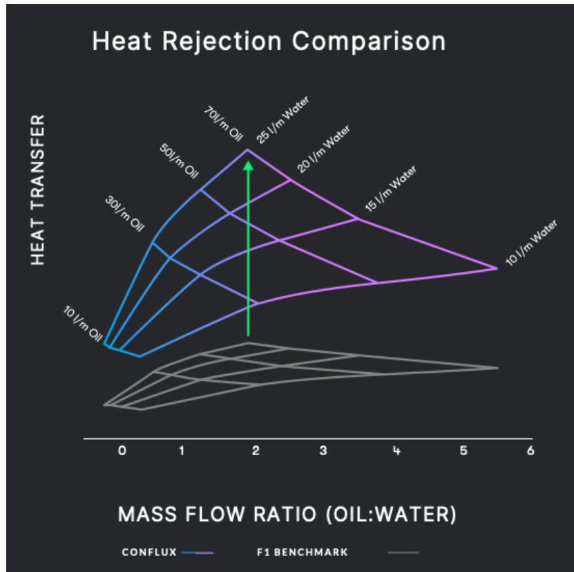
ABOVE: This table shows the heat rejection of Conflux Technology's first patented design compared with a traditionally manufactured F1 benchmark heat exchanger.
